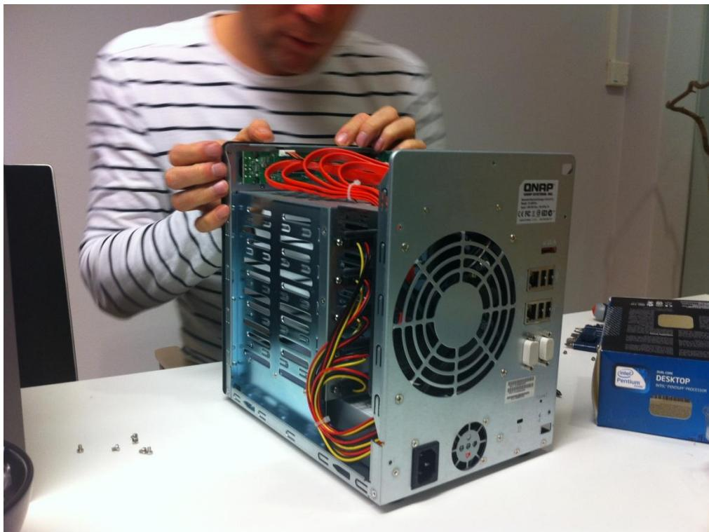
2. Take off the backend...don't forget to loosen the fan connector
