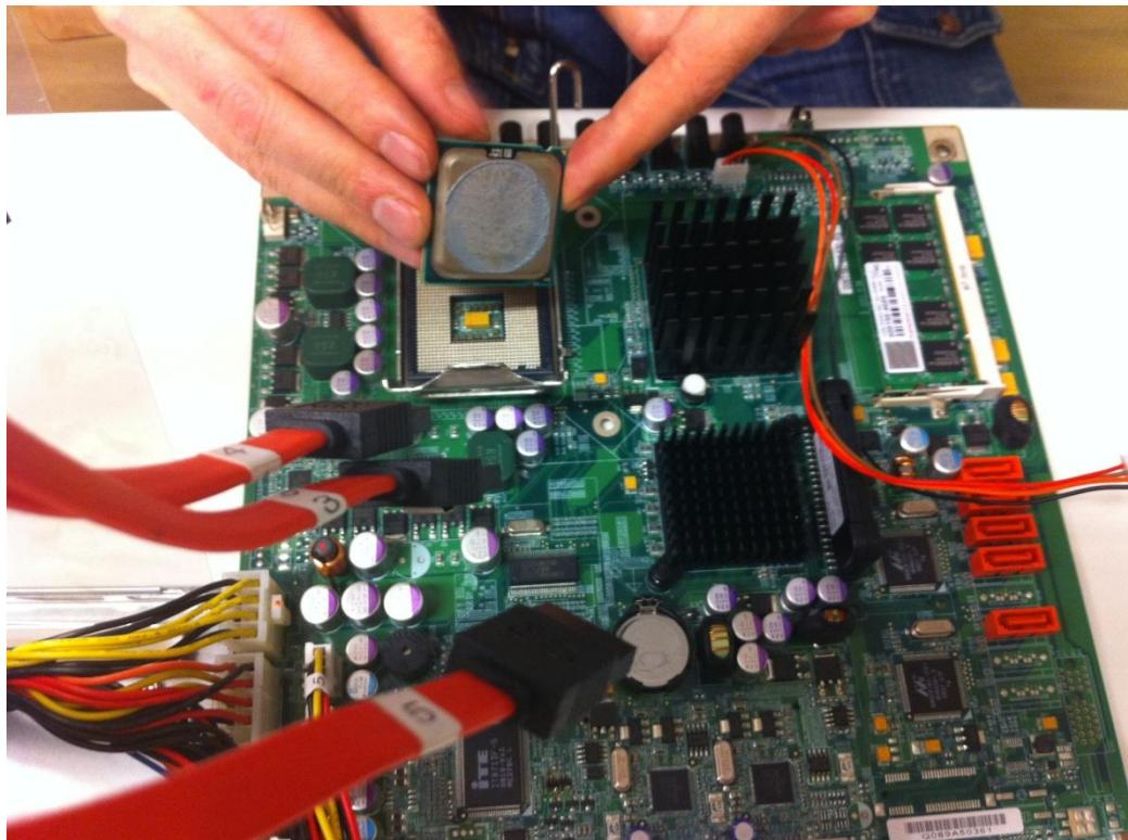
6. Put the new CPU in place and fasten the new intel stock heatsink, be careful not to bend the motherboard....and wash your hands before you touch the back of the motherboard or wear gloves
