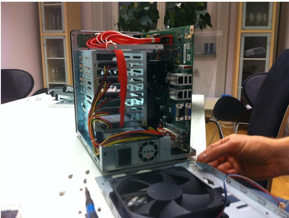
3. Disconnect the SATA connector on the motherboard end
